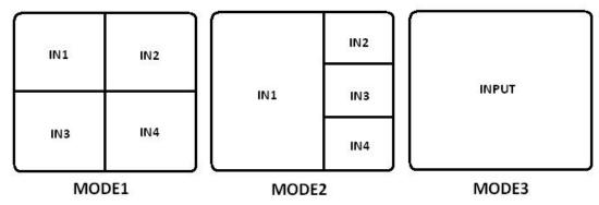
**MODE1:** The quad multi-viewer divides the four HD input to the same size and display on one screen. And now switch the input button on front panel or IR remote, the HDMI output audio will Corresponding to the selected input source.
