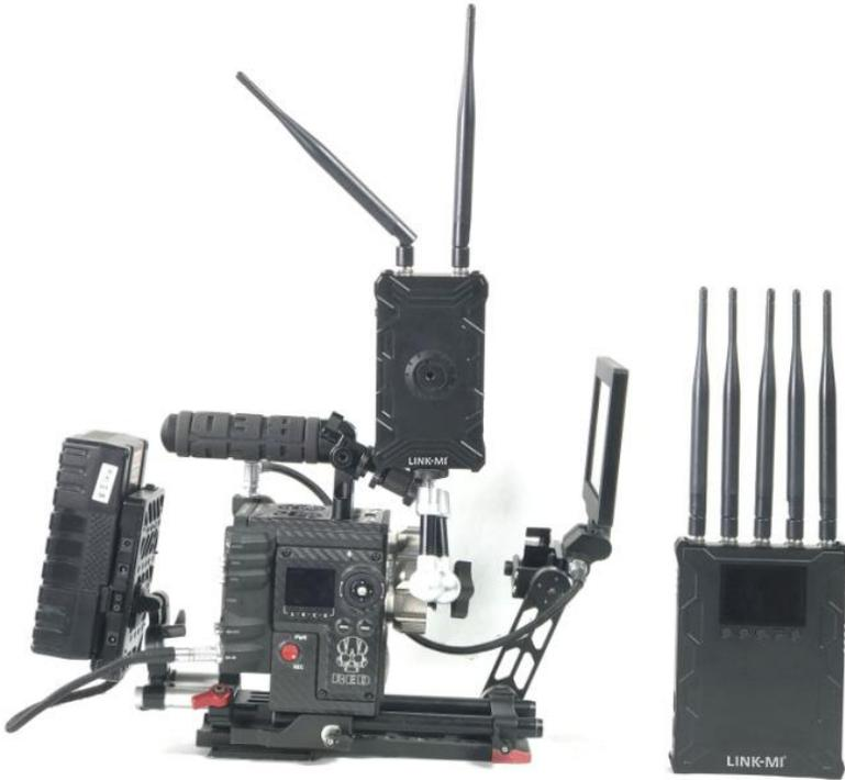
LINK-MI LM-WX1000 is main consist of one transmitter(TX) and one receiver (RX).
