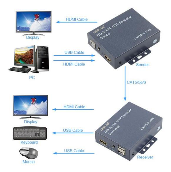
Note: This extender supports independent digital audio. If you do not need, you can connect it with the HDMI line to output video and audio.
