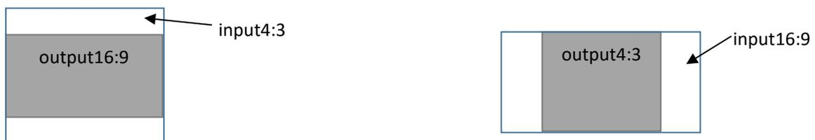
"**Center**" mode is not scaling and processing the input video, and directly output the original video to the middle position. If the input resolution is less than the output video resolution, then the picture is centered and around fill black-edged; if the input resolution is larger than output video resolution, then cut off the video and output to the middle position.
